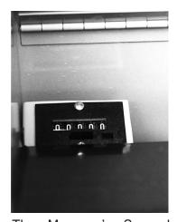
The Manager's Second Counter is positioned under the Safety Feed Ramp, and does not interfere with the Token feed to the Rotary Hopper.
